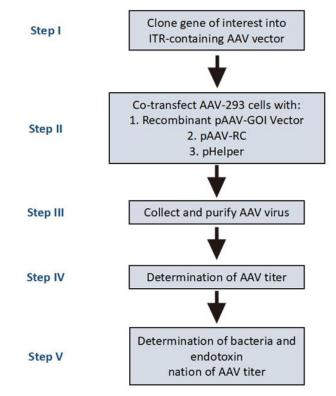
Figure 4. AAV packaging experiment flow chart.
